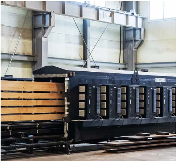
Microwave Drying Technique: This method reduces drying time while preserving the wood's integrity, minimizing deformation risks.
